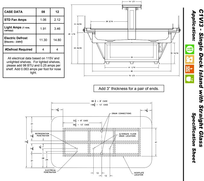
Type I refrigerator, intended for use in an area where the environmental conditions are controlled and maintained such that conditions do not exceed 75 deg F and 55% relative humidity. Kysor//Warren, whose policy is one of continuous improvement, reserves the right to change at any time, specifications, design or prices without incurring obligation. Dual -Jet and Air Defrost are registered trademarks of Kysor//Warren.
