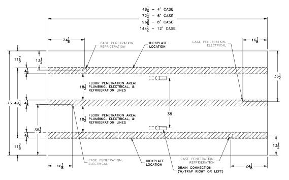
Type I refrigerator, intended for use in an area where the environmental conditions are controlled and maintained such that conditions do not exceed 75°F and 55% relative humidity. Kysor//Warren®, whose policy is one of continuous improvement, reserves the right to change at anytime, specifications, design or prices without incurring obligation. Dual-Jet® and Air Defrost® are registered trademarks of Kysor//Warren®.
