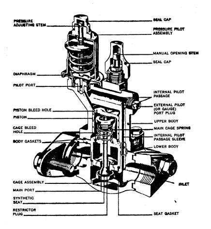
The illustration above shows the basic internal components common to the EPR series and its many pilot combinations. While other models may vary somewhat in construction and pilot configuration, they all operate on a similar principle.
