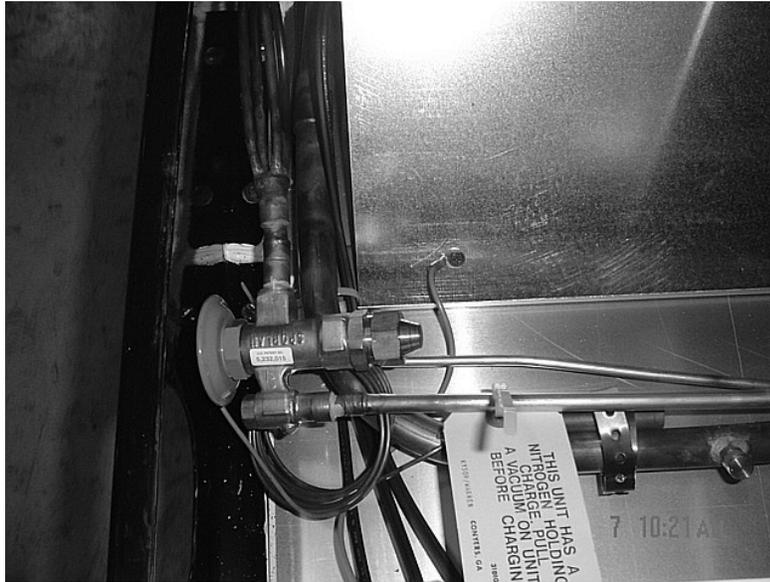
1. Remove wire racks and bottom display pans to gain access to the expansion valve.
