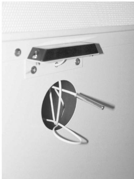
1. Remove the screws securing the digital case temperature display to the case.
