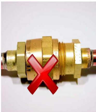
Two Threads Showing
