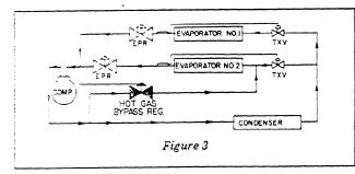
in many applications, an evaporator pressure regulator (EPR) does an excellent job of maintaining evaporator temperature control as loads are reduced. In other cases, the use of an EPR, when preset, compensated by air, by an electric motor, or by a temperature public causes, or may encounter a greatly reduced evaporator load. Below the compressor unloader steps or when
