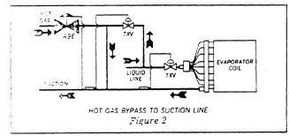
As the load decreases, the suction pressure decreases slightly. "Le Type A9E regulator, sensing the decreased outlet ressure, opens slightly to meter hot gas through the regulator to the suction. To remove the superheat from the bypassed gas, a liquid injection valve should be installed epposite the A9E regulator.
