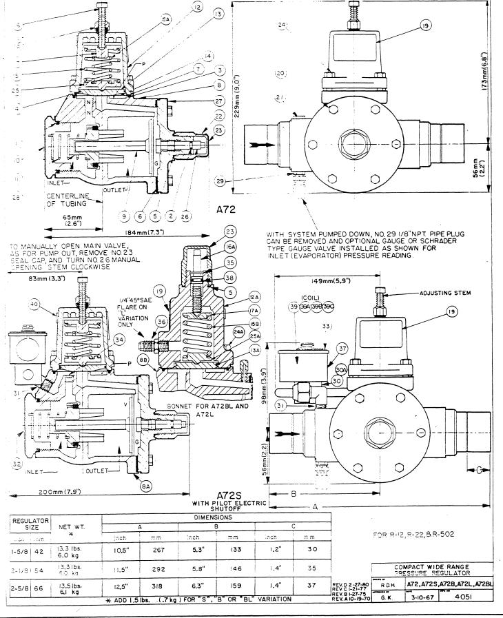
TO RAISE PRESSURE SETTING OF VALVE, LOOSEN SEAL NUT
