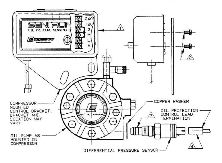
his page describes an electrical check for the Copeland Sentronic oil pressure module and sensor installed in an ir-conditioning or refrigeration system.
