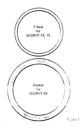
(tetraseal for (S)ORIT-12 and -15; composition gasket for (S)ORIT-20), and I copper flare gasket for the (S)ORIT-20.
