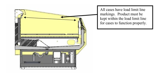
Do not place product in cases until it is at proper operating temperature. Air discharge and return flues must remain open and free of debris or obstruction at all times to provide proper refrigeration and air current performance. Do not allow any product, signs, debris, etc. to block these grilles. Do not use any non-approved shelving, display racks or any accessory that could hamper air current performance.
