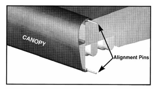
Align the case front rails with a single alignment pin sliding the pin across the joint into the adjoining front rail. It may be necessary to loosen the screws holding the front rail to aid in the alignment process. The screws should be tightened after the front rails are aligned.
