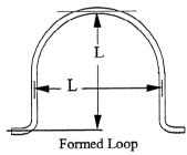
In order to compensate for the expansion of the tubing, it is necessary to estimate the amount of expansion and then provide offsets or loops in the refrigerant piping. As a general rule, medium temperature lines will expand approximately 1-1/2" for each 100' and low temperature lines approximately 2" for each 100' of tubing. Normally, in a supermarket, the area to be most concerned with is the straight line distance from the fixture to the main access pit in or near the motor room.
