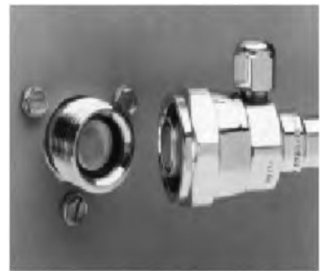
Clean and Lubricate Couplings
