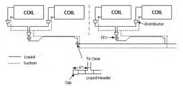
NOTE: All 4 FT and 6 FT cases are single coil and single valve piping. Our standard 8 FT and 12 FT cases have 2 coils and 2 TXV (expansion valves). Custom orders on 8 FT and 12 FT cases that have 1 valve, the valve must be electronic and the case must have a case controller.
