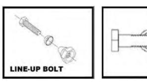
hole pattern. Place the special T-nut washer on the 3/8" machine bolt with the hollow section away from the bolt head. Tighten the 3/8" bolts with nut washer into the T-nuts alternately until cases are pulled up tight and the joint is completely sealed. (Reasonable care should be exercised in this procedure to prevent end frame distortion.) Assist pulling case up tight by bumping from opposite end of case or by using pry bar.
