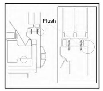
B. Tighten these important screws with approx. 30Nm torque.
