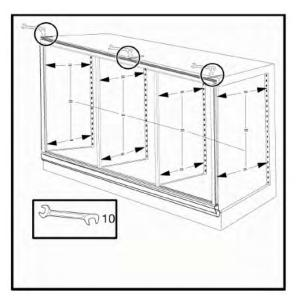
B. The fronts of the "frame bottom profile" and "support profile" must be flush.
