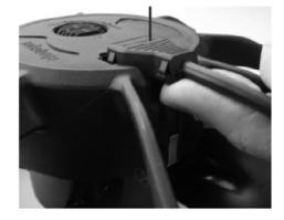
ty across the speed selection and L1 pins with the common lead on the L1 pin. Both measurements should have a value of M $\Omega$ 's (typically 2-3M $\Omega$ ). If either reading is zero or infinity, replace the fan.
