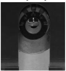
4. Push up on tabs and pull the indicator tab away from the angle dial.
