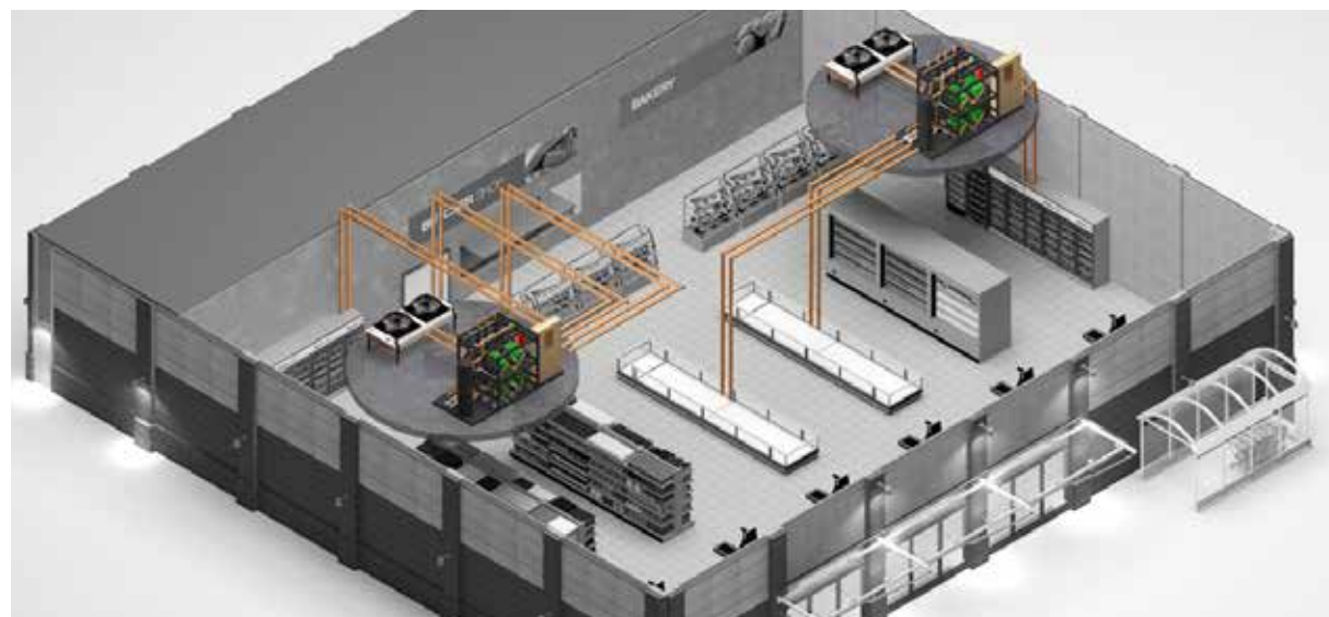
Figure 1-2. Example of a distributed Refrigeration System
