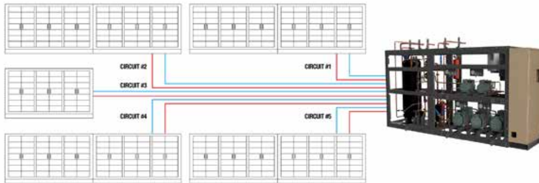
Figure 1-17. Piping for a Circuit
