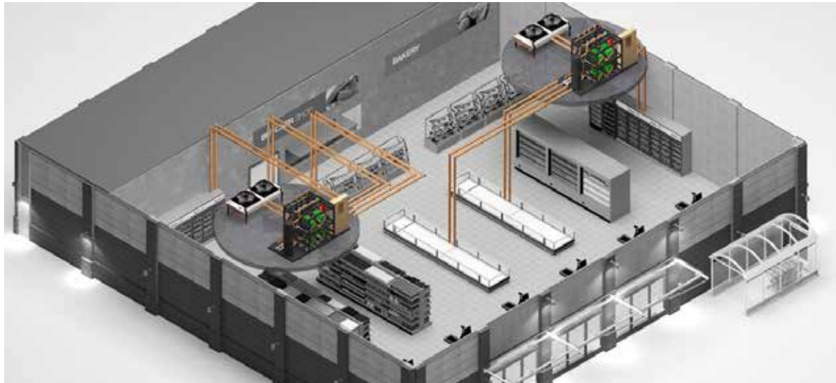
Figure 1-2. Example of a distributed Refrigeration System
