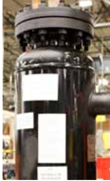
Figure 1-4. Coalescing oil separator
