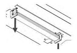
4. Push up on tabs and pull the indicator tab away from the angle dial.
