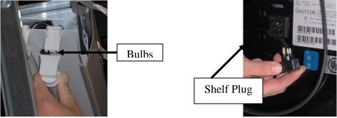
Note: The fluorescent bulb is capable of lighting even if the bulb and shelf power cord are not completely seated.
