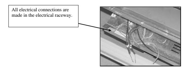
The wires are clearly identified for termination purposes as follows:
