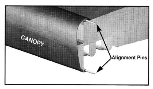
the adjoining front rail. It may be necessary to loosen the screws holding the front rail to aid in the alignment process. The screws should be tightened after the front rails are aligned.
