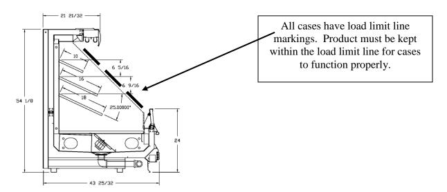
Do not place product in cases until it is at proper operating temperature. Air discharge and return flues must remain open and free of debris or obstruction at all times to provide proper refrigeration and air current performance. Do not allow any product, signs, debris, etc. to block these grilles. Do not use any non-approved shelving, display racks or any accessory that could hamper air current performance.
