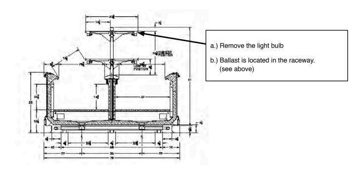
WARNING! It is imperative that the pins of the bulbs and the shelf power cords be completely seated in their respective lamp holder or receptacle. If they are not completely seated, an electrical arc could occur which will cause the lamp holders or the shelf light receptacles to melt and become an electrical hazard. Care must be taken during cleaning, product stocking and re-lamping processes to insure that the bulbs and shelf cords are not dislodged.
