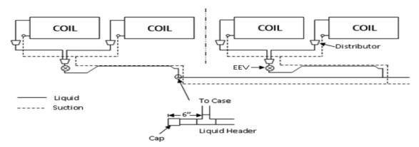
NOTE: All 4 FT and 6 FT cases are single coil and single valve piping. Our standard 8 FT and 12 FT cases have 2 coils and 2 TXV (expansion valves). Custom orders on 8 FT and 12 FT cases that have 1 valve, the valve must be electronic and the case must have a case controller.
