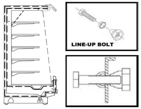
bolt head. Tighten the 3/8" bolts with nut washer into the T-nuts alternately until cases are pulled up tight and the joint is completely sealed. (Reasonable care should be exercised in this procedure to prevent end frame distortion.) Assist pulling case up tight by bumping from opposite end of case or by using pry bar.
