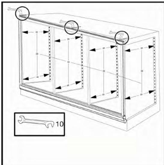
B. Tighten these important screws with approx. 30Nm torque.
