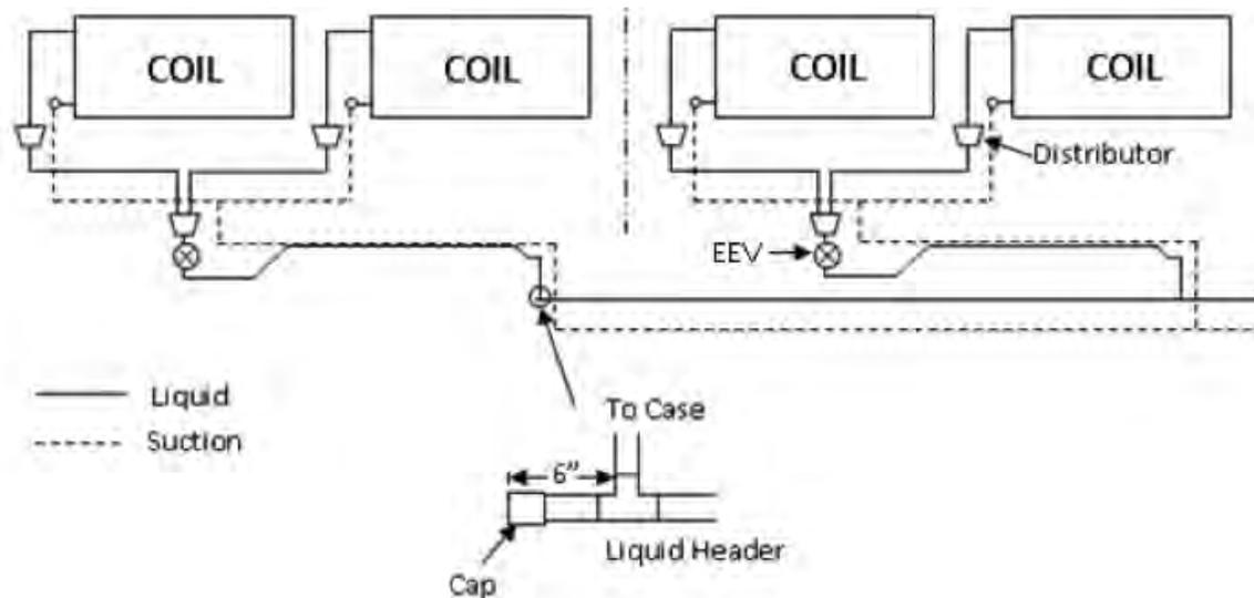
NOTE: All 4 FT and 6 FT cases are single coil and single valve piping. Our standard 8 FT and 12 FT cases have 2 coils and 2 TXV (expansion valves). Custom orders on 8 FT and 12 FT cases that have 1 valve, the valve must be electronic and the case must have a case controller.
