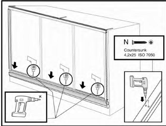
B. The fronts of the “frame bottom profile” and “support profile” must be flush.
