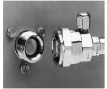
Clean and Lubricate Couplings
